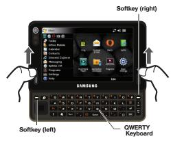
The built-in QWERTY keyboard supports quick and easy text input, just as you would when using a computer's keyboard. Mondi also provides an onscreen virtual QWERTY keyboard that functions in the same fashion.
